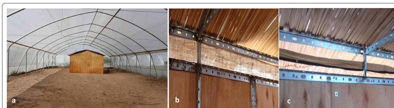
Fig. 1 a Pictorial presentation of a semi-field system (27 m × 11 m), including an experimental hut made of plywood with a grass thatched roof (6.5 m × 3.5 m). b Application of an eave screen secured on the eave gap of the experimental hut using aluminium wires to ensure complete coverage of the eave gap ( c ) and eave strip secured on the eave gaps of the experimental hut using aluminium wires to ensure equal distance (2.5 cm) above and below the eave fabric
