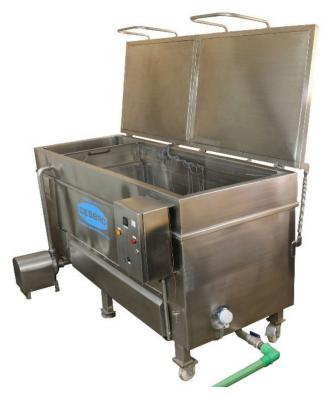
**Figure 1.** Insulated stainless steel hot water treatment machine. Lids were only in use during the water heating process and opened once the treatment started.
