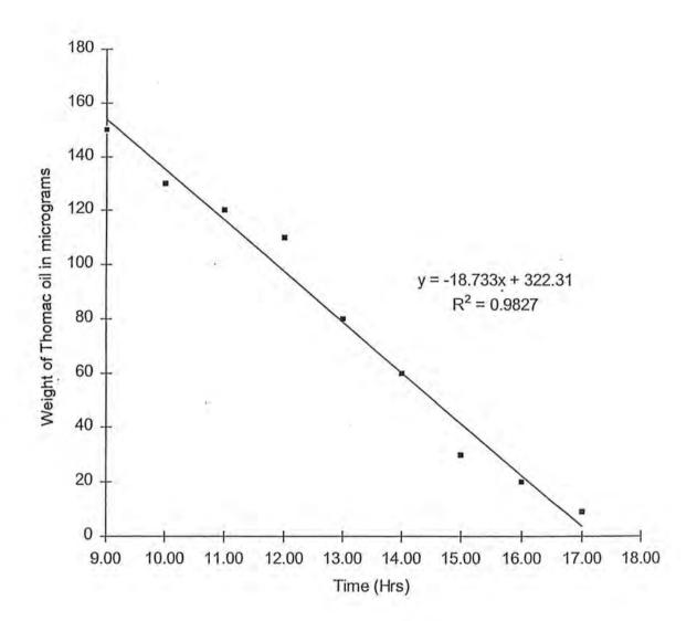
Figure 14. Release rate of 100 μg of (E)-β-farnesene
