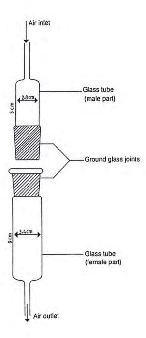
Figure 2. Glass chamber for placing test material (plant volatiles)
