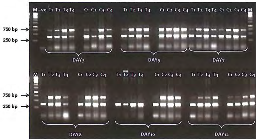
Figure 14. Verification of gene-knockdown. The PCR products were separated on a 1% agarose gel electrophoresis. M: 1Kb DNA ladder, Fermentas.
