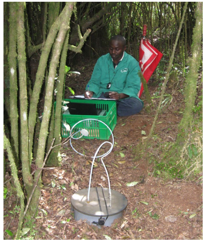
Chamber placement for CO 2 gas measurement in avocado-agro-forestry systems (left), and chamber based CO 2 gas measurements in Taita hills natural forests. Photos by: Crispus Mugambi/ CHIESA
