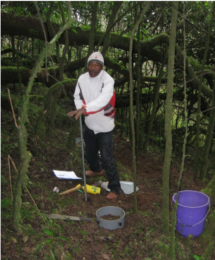
Chamber placement for CO 2 gas measurement in avocado-agro-forestry systems (left), and chamber based CO 2 gas measurements in Taita hills natural forests. Photos by: Crispus Mugambi/ CHIESA
