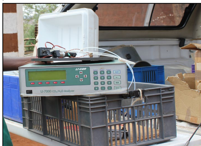
Clockwise from left: A LICOR 7000 CO 2 /H 2 O analyzer, used for field measurements of carbon dioxide gas emissions from the soil; a mini laptop data logger that connects to and receives data from the LICOR analyzer; a minimum/maximum thermometer for measuring surface temperatures during gas sampling; and one of several calibration gas (401 ppm pure grade CO 2 ) cylinders used to calibrate the LICOR analyzer during sampling. Photos by: Kelah Kathure/ CHIESA
