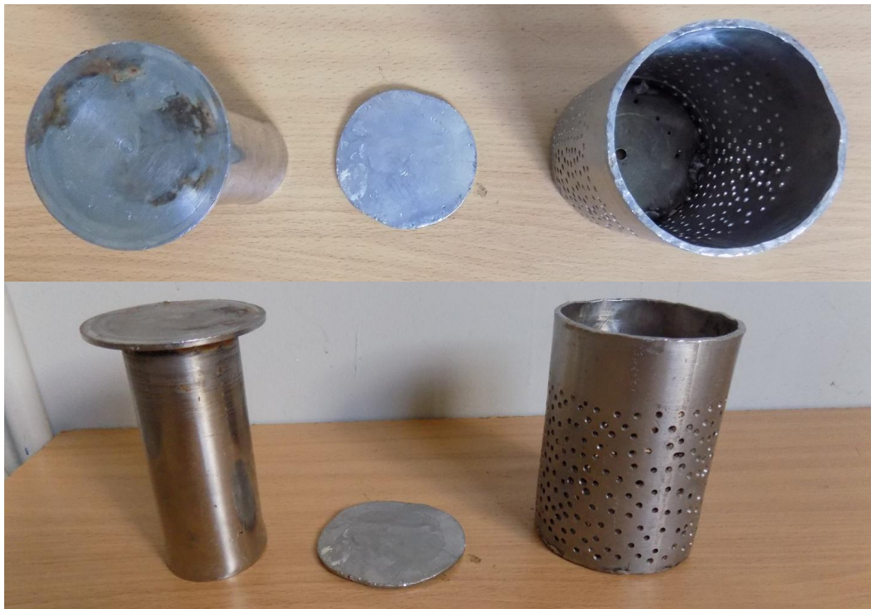
Figure 3.3. Sugarcane juice extractor; piston, circular plate and perforated container
