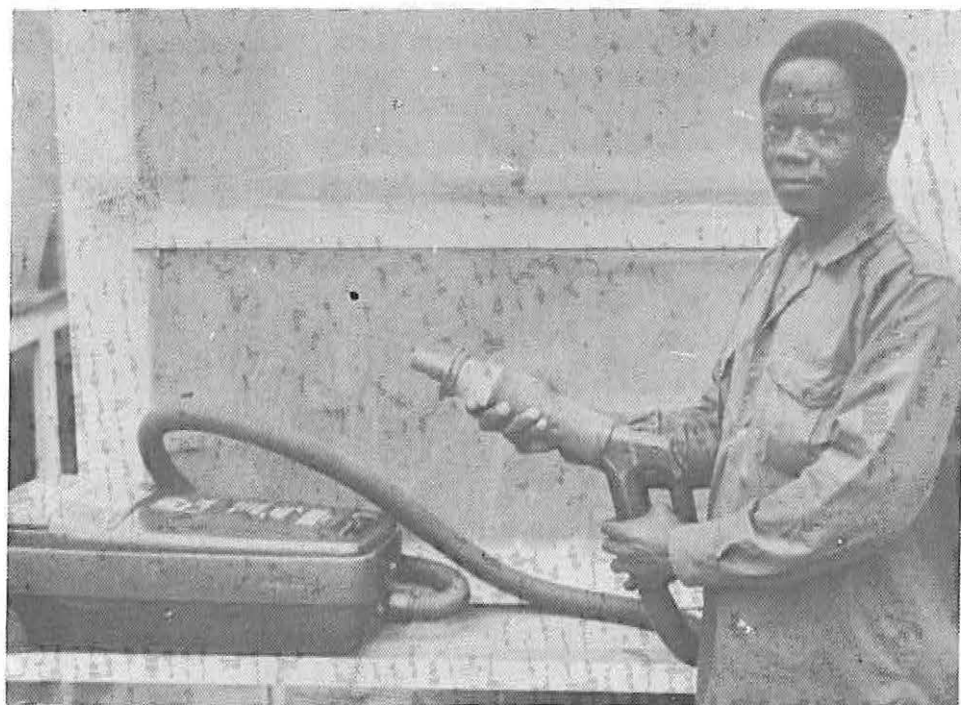
Fig. 7. Vacuum attachment for collecting leafhoppers from the nymphal rearing cage
