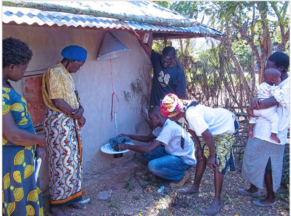
Fitting of a solar-powered mosquito trapping system (SMoT) in a homestead on Rusinga Island, western Kenya.
