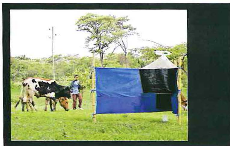
NGU tsetse trap, one of the landmark developments of icipe
