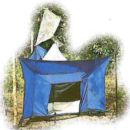
The S3 trap, one of several traps currently being tested in Ethiopia for catching Glossina morsitans submorsitans . This species avoids most current trap designs.
