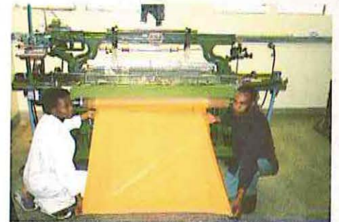
The first silk cloth produced by the Commercial Insects Megaproject from African cocoons comes off a simple purpose-built powerloom.
