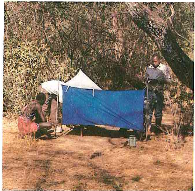
Installing and inspecting the ICIPE NG2B trap in Nguruman. These traps when placed at a density of 2–3 traps/km 2 have effectively lowered the tsetse population in the area to 98–99% of pre-trapping levels. The tin can on the right holds the odour bait of cow urine and another container the acetone bait.
