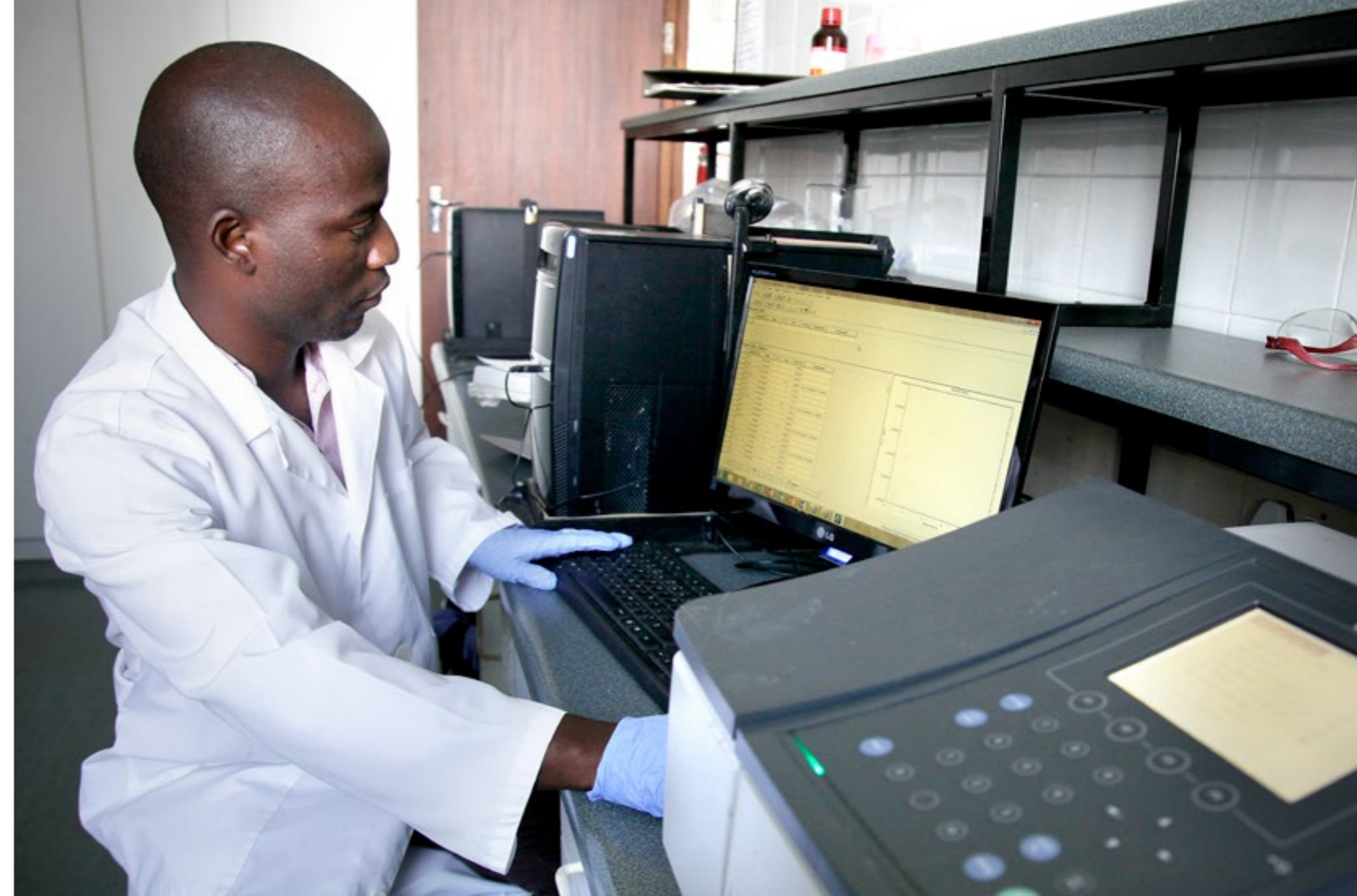
Dr Learnmore Mwadzingeni, a post-doctoral fellow at the ACCI, works on a UV 1800 spectrophotometer, used for analytical assessment of organic acids.
