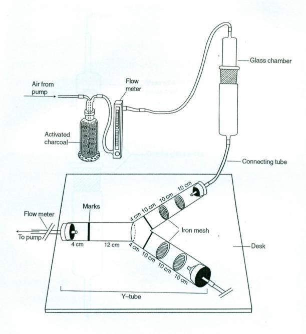
Figure 1. A schematic representation of the Y-tube olfactometer (Ngi-Song, 1995)
