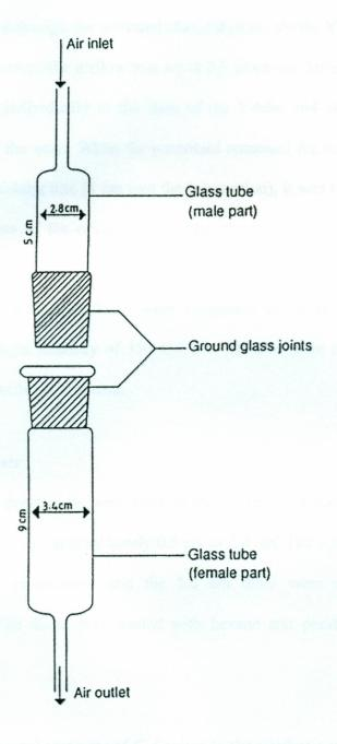
Figure 2. Glass chamber for placing test material (plant volatiles)
