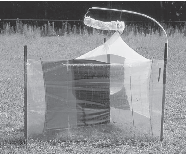
Fig. 2. Side view of the Nzi trap enclosed in a continuous wall of transparent Rentokil fly control adhesive film in Ontario. A Dragonfly® octenol lure hangs at the back corner.
