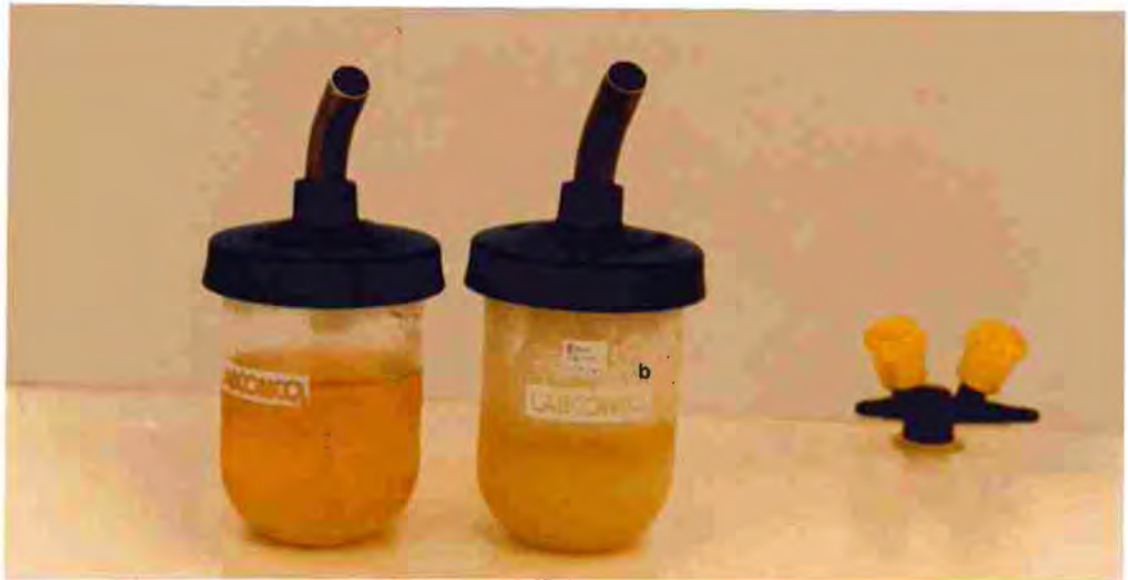
Plate 4a: A virtis ® freeze drier with freeze drying bottles containing plant extracts. b: Labconco ® freeze drying bottles containing frozen extracts before attachment to the freeze drier.
