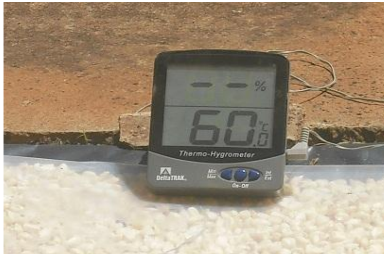
Plate 4.2: Temperature measurement with a thermo-hygrometer during solar disinfestation
