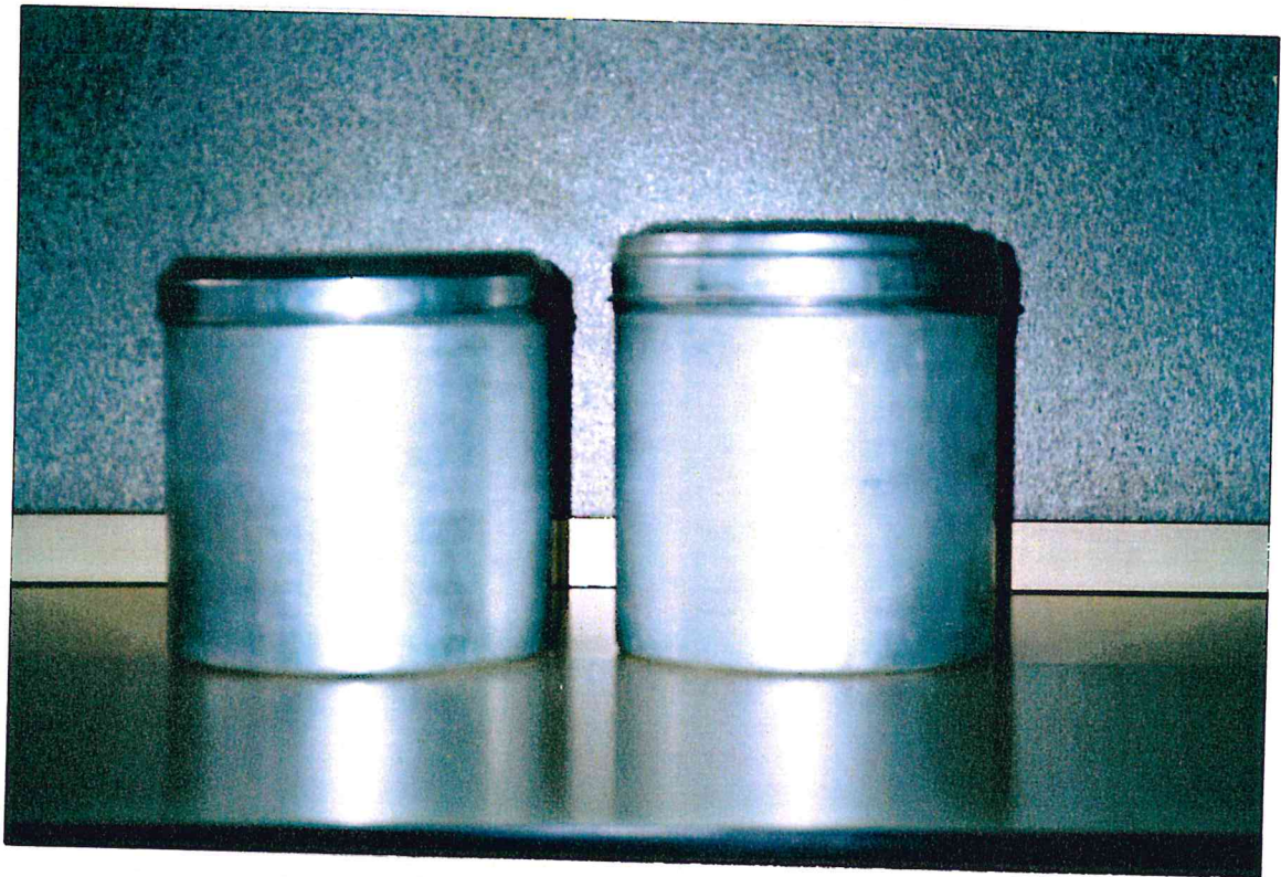
Plate 3.2. Aluminium cans in which parasitized replete A. variegatum nymphs were kept till the emergence of the parasitoids (height = 20cm, diameter = 20cm)
