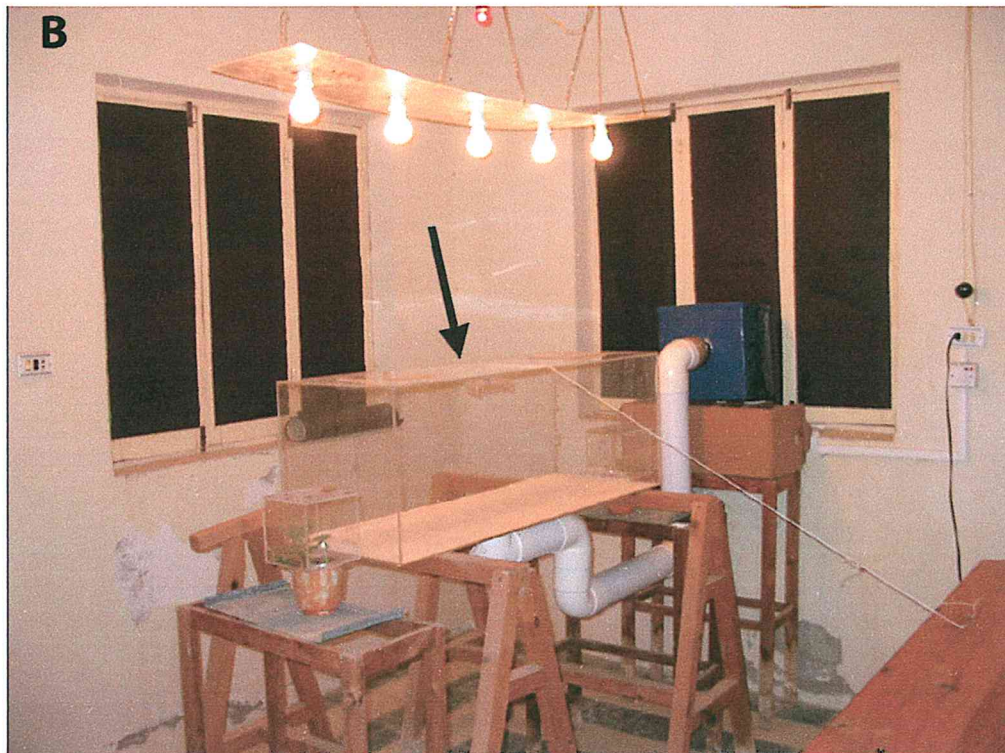
Plate 5. Flat-bed (A) and two-choice (B) wind tunnels (arrows)
