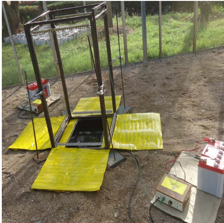
Figure 10: A complete set up of a square of e-nets
