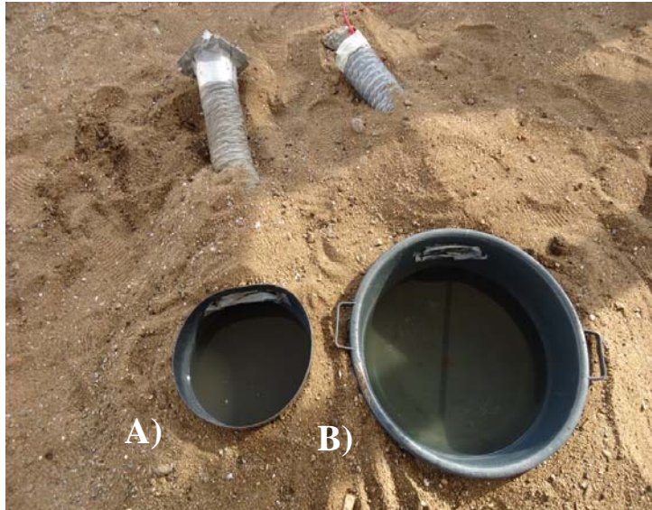
Figure 19: A) The prototype OviART gravid trap, B) The OviART gravid trap with bigger basin
