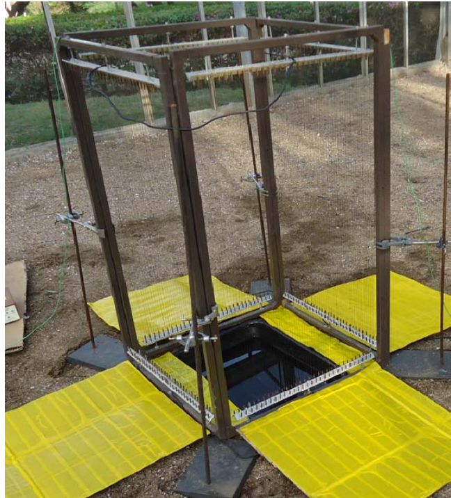
Figure 6: A complete square of four electrocuting nets surrounding an artificial aquatic habitat. Yellow sticky boards serve as collection device for stunned mosquitoes.
