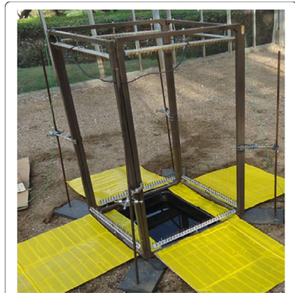
Figure 5 A complete square of four electrocuting nets surrounding an artificial aquatic habitat. Yellow sticky boards serve as collection device for stunned mosquitoes
