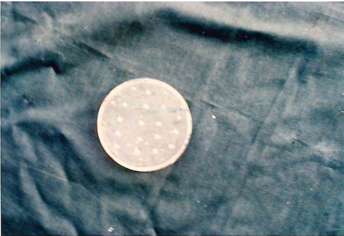
Plate 1. Plastic Petri-dishes showing perforations through which water passes by capillary action
