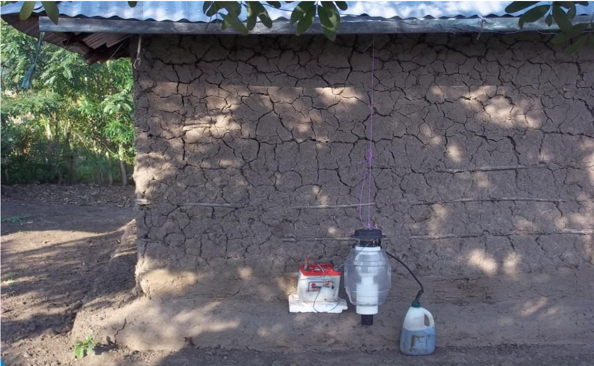
Figure 1: A picture of a trapping system baited with the Mbita odour blend augmented with carbon dioxide produced by fermentation of 250 g of molasses using 17.5 g of dry yeast mixed with 2 L of water. Carbon dioxide was produced in a plastic container and delivered into the MM-X trap through a silicon tubing. The trapping system was deployed outside the bedroom under the overhanging roof of a village house to collect outdoor biting mosquitoes at night (18:30 ó 06:30 h). Photograph: C.K. Mweresa
