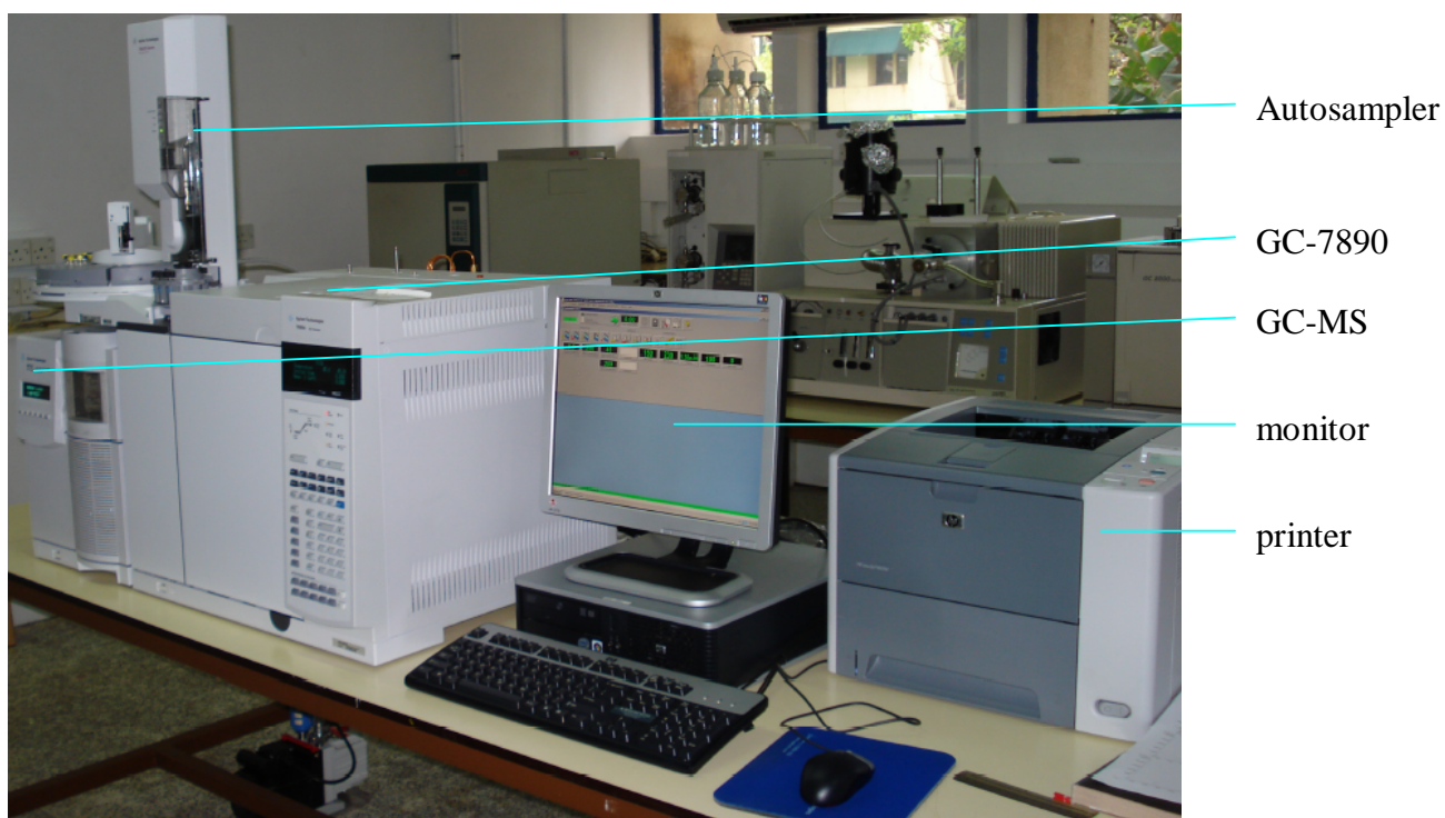
Plate 5.2 Gas chromatography linked mass spectrometer equipped with an autosampler and coupled to a HP monitor used for GC-coupled mass spectrometric analyses of volatile collections.
