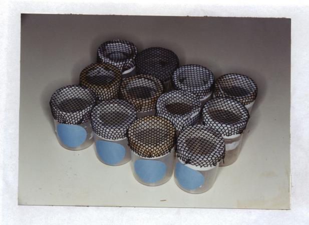
PLATE 2 Transparent plastic tubes used for holding tsetse singly during transmission of *T. congolense* from flies to mice. The top side of the tubes is covered with netting material.
