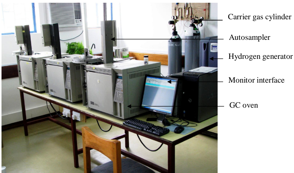
Plate 2.7 Gas chromatographs attached with autosamplers on the injector port and connected to a HP (Dell) monitor and PC (Photography by F. Kimbokota).
