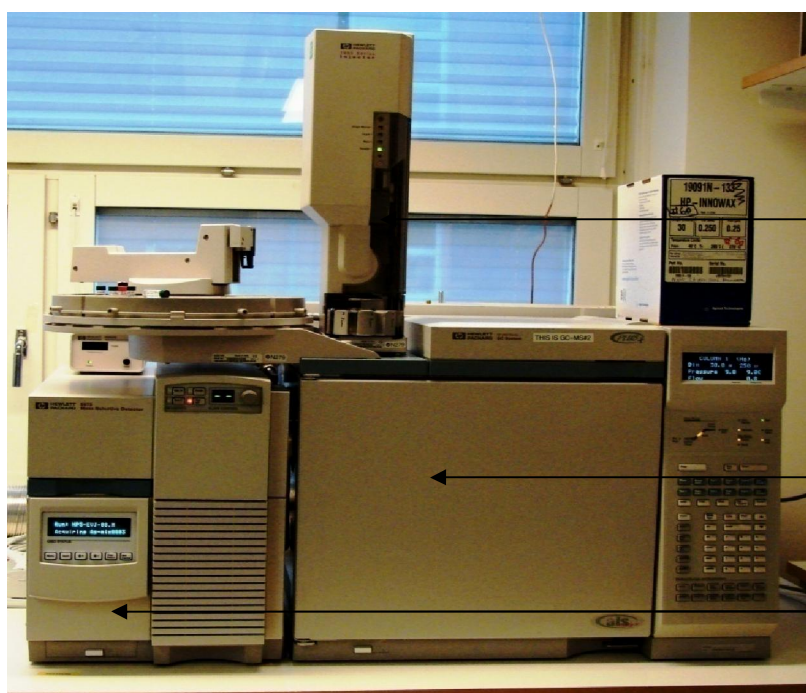
Plate 2.10 HP 6890 series GC-MS with an attached autosampler used for chemical identification of volatile components (Pheromone group – University of Lund, Sweden).
