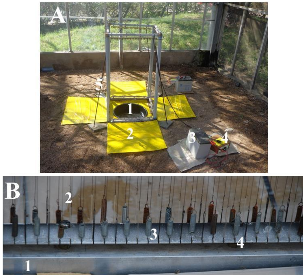
Figure 6.2: Square of electrocuting nets for analysing pre-oviposition behaviour of gravid mosquitoes. (A) Overview of the set-up: (1) artificial pond created by sinking a plastic tub filled with water into the ground, (2) sticky boards for collection and preservation of electrocuted mosquitoes, (3) 12 V battery, (4) spark box, (5) clamp and stand. (B) Close-up of electrocuting net: (1) aluminium frame (2) fish line wire (3) spring (4) aluminium bar.
