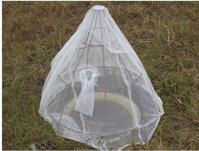
Figure 2.1: Standardized field test set up. Netting-covered emergence trap on top of artificial pond.
