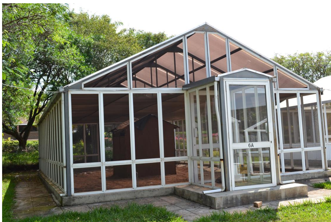
Figure 7.1: Semi-field system showing artificial hut constructed at the centre of the semi-field system
