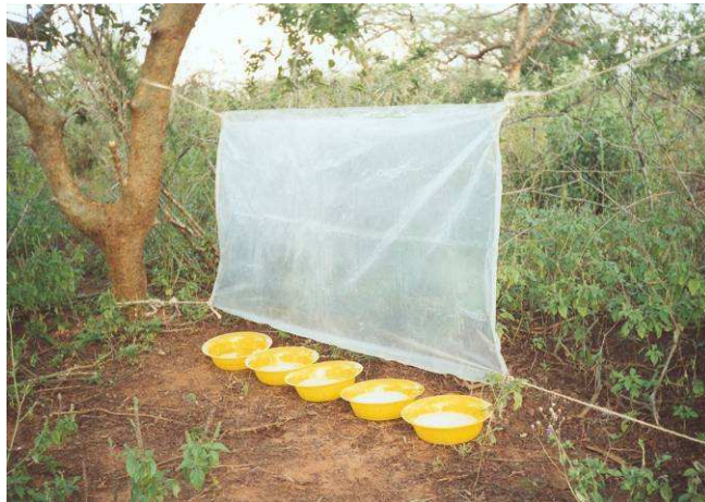
Figure 2.2: Flight intercept trap used to sample Histeridae predating on bark-boring Coleoptera. Insects collected in soapy water in the yellow troughs were transferred into absolute ethanol every 12 hours.
