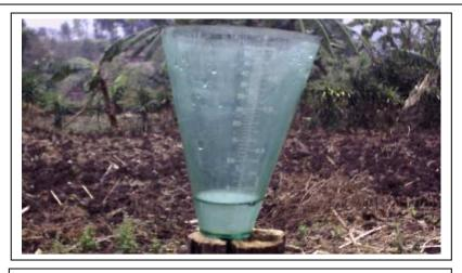
Plate 3.6: Rain gauge for recording rainfall
