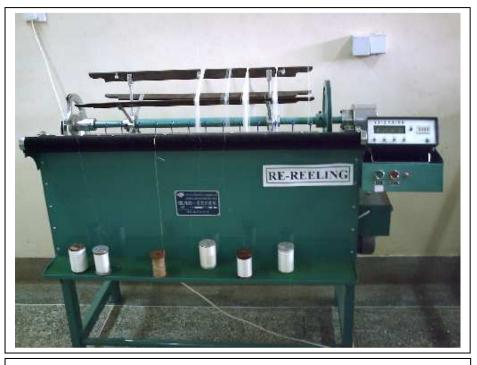
Appendix 11: Winding frame reel and serigraph for tenacity and elongation measuremement
