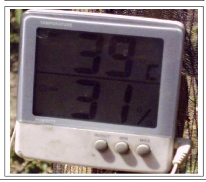
Plate 3.5: Digital hygrothermometer for recording temperature and RH
