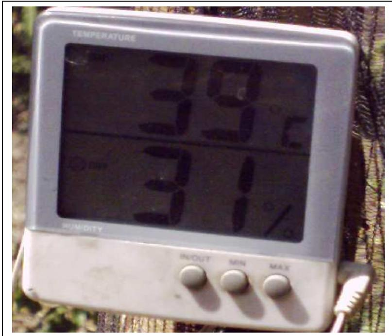
Plate 3.5: Digital hygrometer for recording temperature and RH
