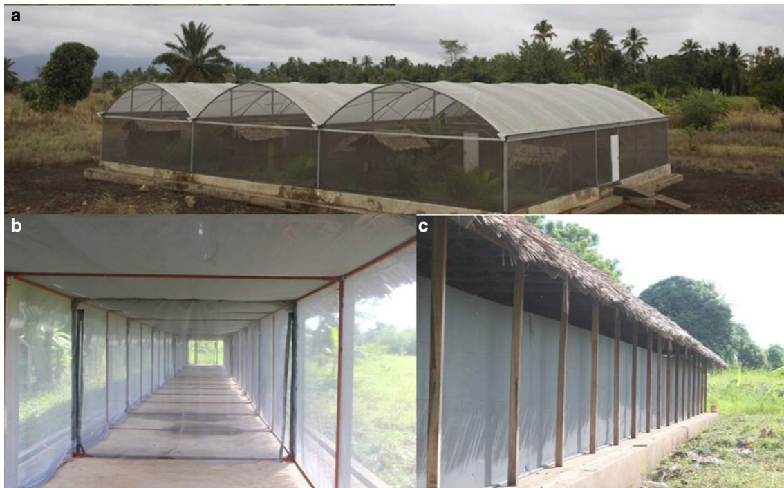
Fig. 1 Pictorial illustration of (IH) semi field cages, a large multi-compartment system; b inside sections of the long, tunnel-shaped screened semi-field system; c outside view of the long tunnel-shaped screened semi-field system
