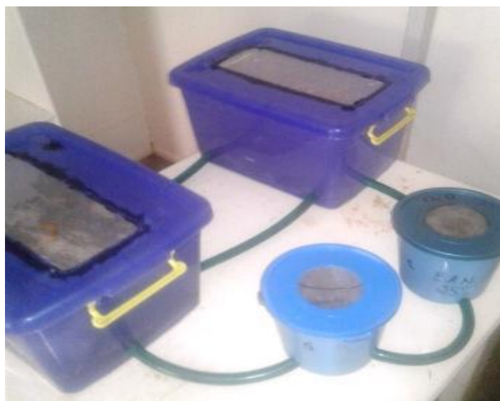
Figure 6-1: Artificial system for maintaining termites in the laboratory
