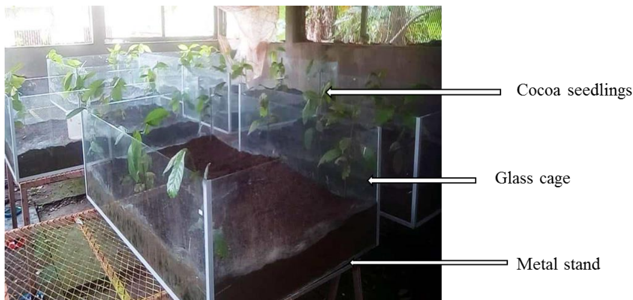
Figure 7-1: Set-up for semi-field trial of the attractiveness of CO 2 -emitting capsules to subterranean termites
