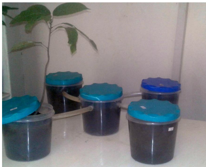
Figure 6-4: Experimental set-up for testing the attractiveness of CO 2 emitting capsules co-formulated with M. brunneum to termites
