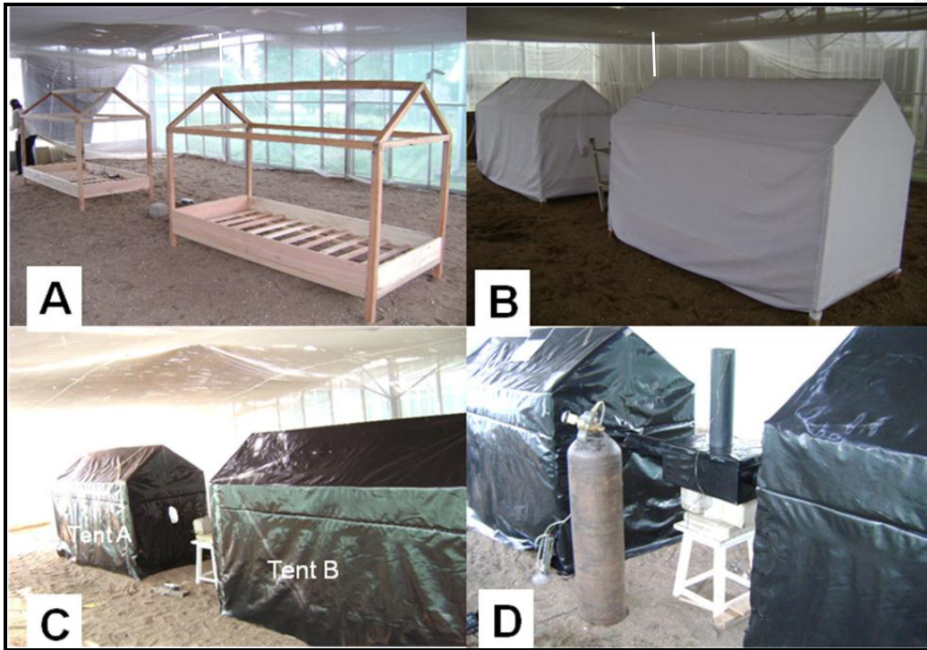
Plate 2: Pictorial view of the experimental apparatus used to study the response of An. gambiae to human emanations and synthetic odours augmented with physical cues. A, wooden framework of the tents; B, tents' framework covered with thick white cotton cloth; C, opaque polythene paper (PCV) overlying the white cotton cloth tent covers; and D, the dual-port olfactometer connected to the two tents.
