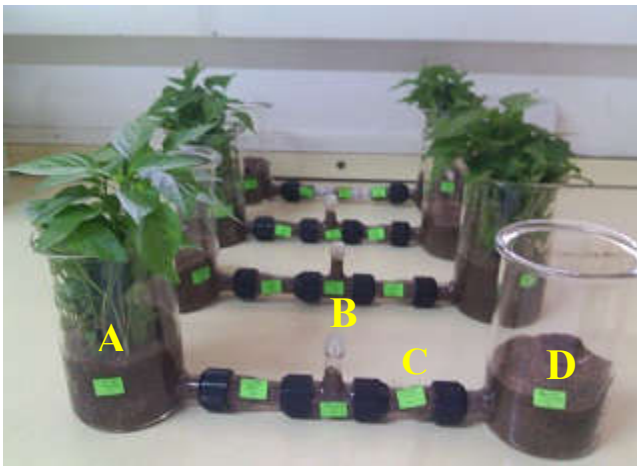
Plate 3.3: Dual choice olfactometer assays to test J2s responses to Capsicum root volatiles and synthetic blends (A) Stimulus chamber, (B) Release arm (C) Connecting arm, (D) Control chamber
