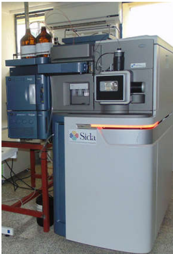
Plate 3.5: Liquid chromatography-quadrupole time of flight-mass spectrometer for analysis of pepper root exudates
