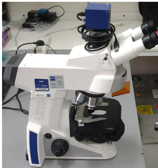
Figure 5: A picture of compound light microscope (Carl Zeiss MicroImaging GmbH 37081, Gottingen, Germany).
