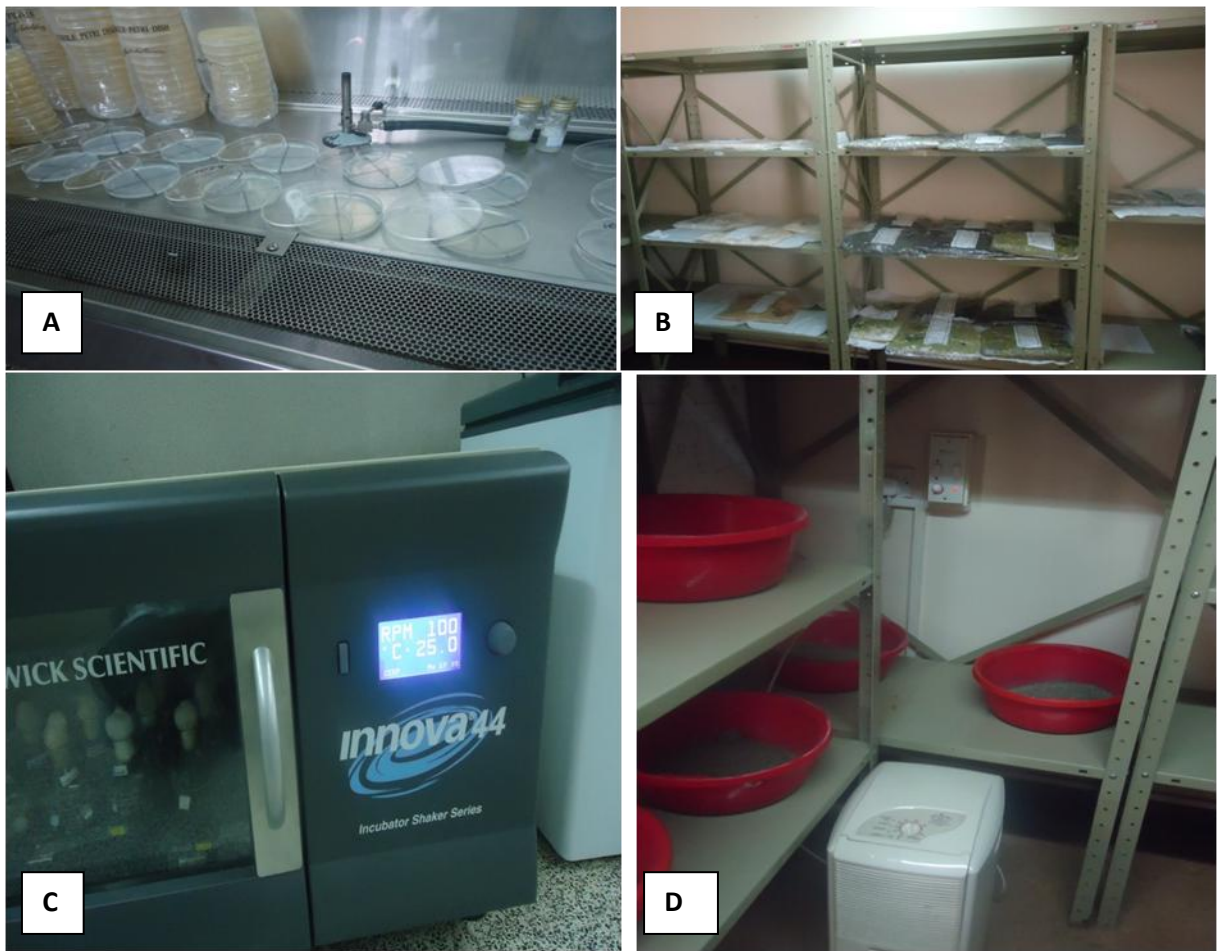
Figure 1. Basic facilities and equipment for small scale mass production of EPF. A) Microbial bio-safety flow hood, B) Dehumidified room for sporulation and drying of inoculated bags, C) Digital incubator shaker for production of blastospores in the liquid phase and D) Plastic bowls for drying shown with an automatic dehumidifier.
