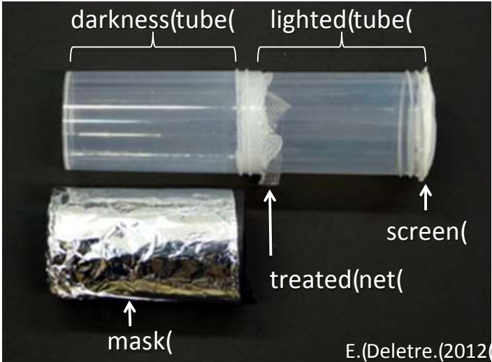
Fig. 1. Apparatus used for the irritant bioassays on B. tabaci .
