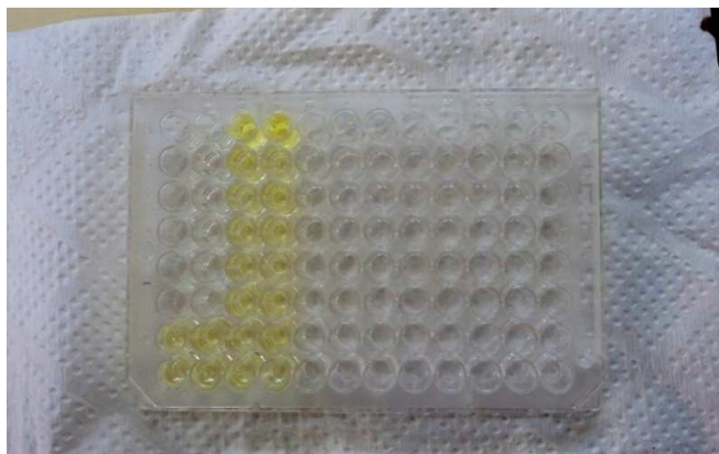
Plate 9. 3: 96-wells plate showing reactions using the DAS-ELISA technique
