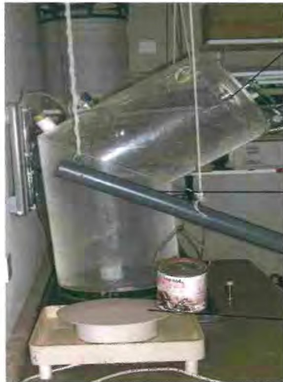
Plate 3.1 Burgerjon spray tower used to spray conidial suspension onto termites
