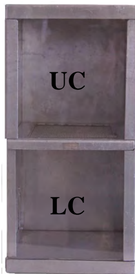
Plate 3.2: Double storey cage (30 x 15 x 15cm) for testing the effect of nymphal volatiles on sexual maturation of immature adults. LC, Lower compartment; UC, Upper compartment.
