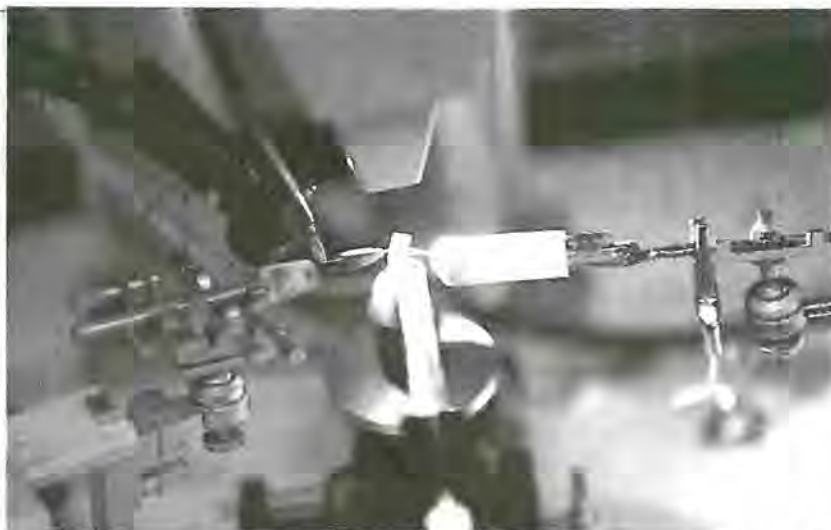
Figure 7. Preparation for single cell recording. The locust is restrained inside a holder with the antennae sticking out. The antenna is placed against a stage to allow for penetration of the cuticle with an electrode when viewed under a stereo microscope ( \times 320 magnification).
