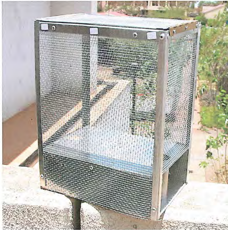
Plate 6. Wire mesh oviposition cage (30 cm x 20 cm x 20 cm)
