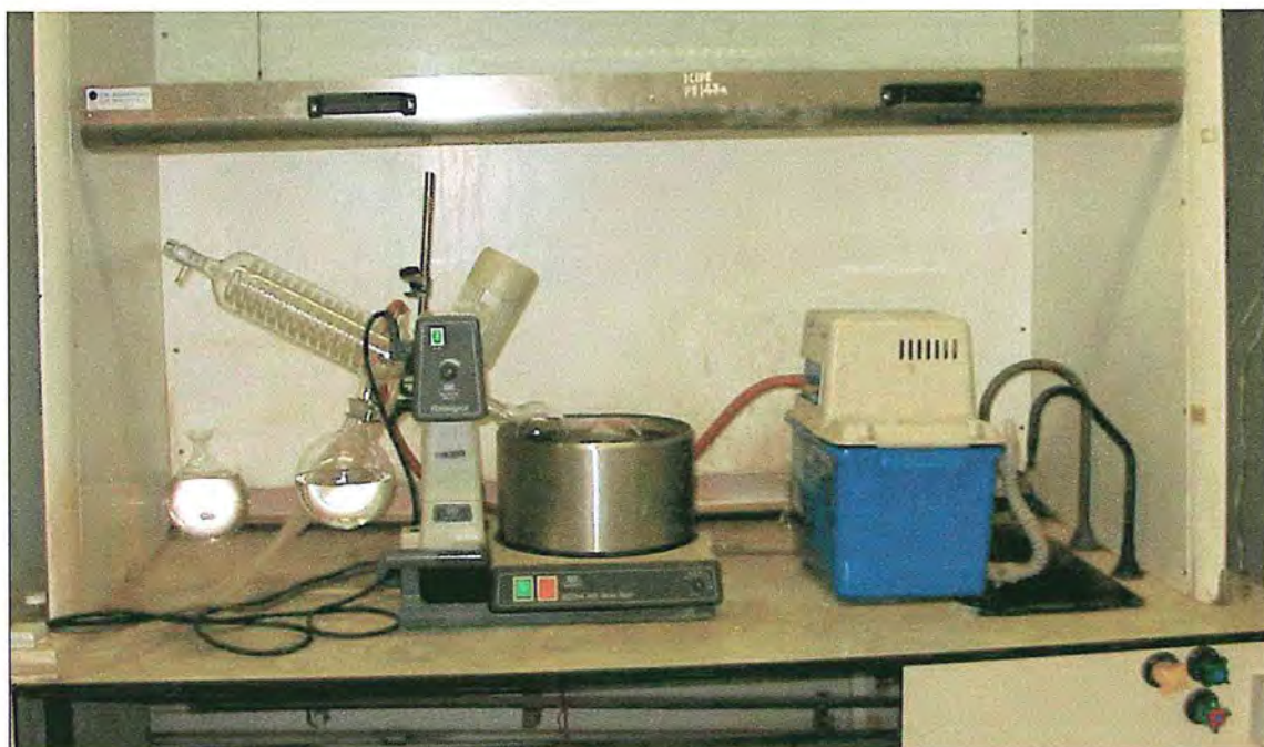
Plate 8. Rotavapor (Büchi 461, water bath, Switzerland)
