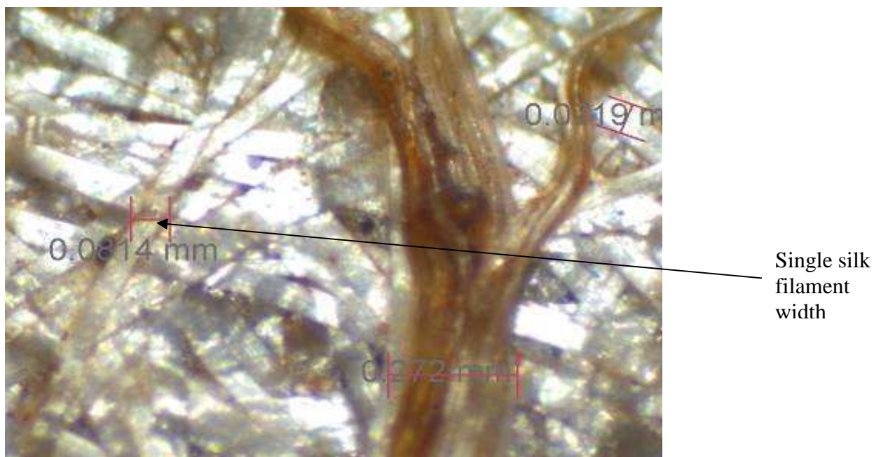
Plate 7.11: A cross section of A. mimosae cocoon showing silk filament width in Millimeters, Magnification: 350
