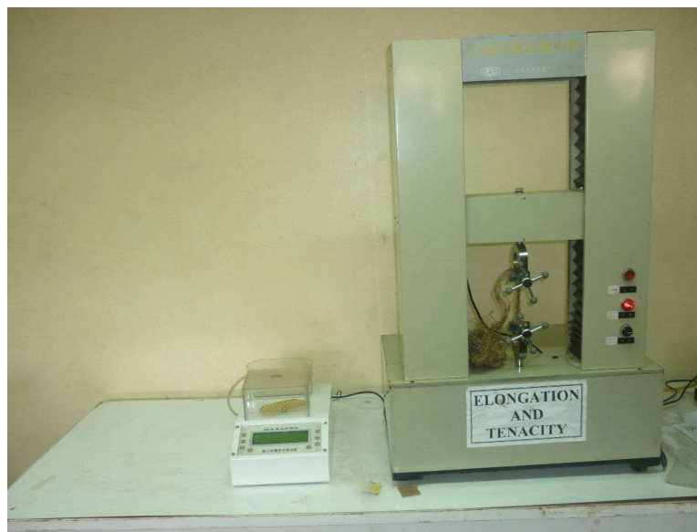
Plate 3.1: Elongation and breaking load testing machine
