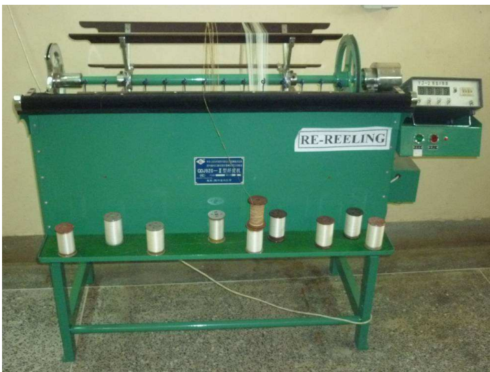
Plate: 7.2: A Sizing reel used to prepare elongation and tenacity test samples
