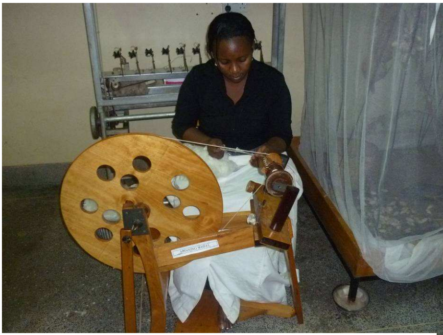
Plate: 7.1: A wooden manual spinning wheel used to spin A. mimosae silk floss
