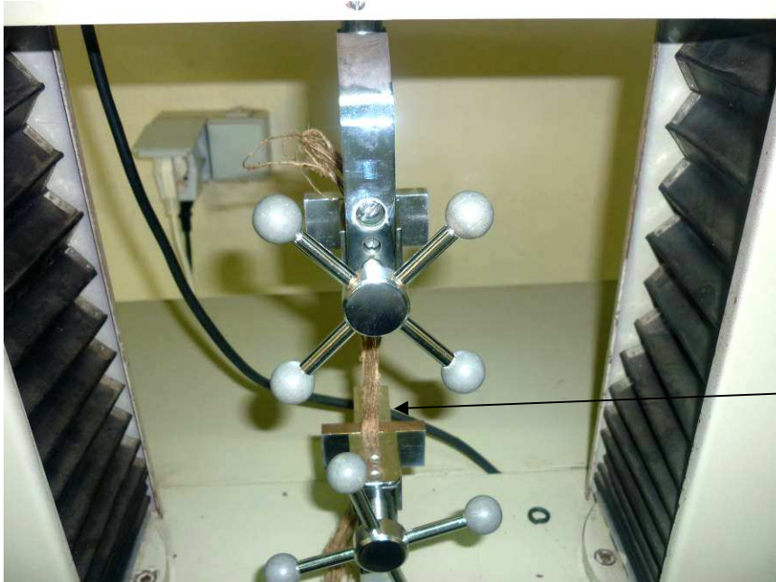
Plate: 7. 3: Argema mimosae silk fibre fixed on serigraph before elongation and tenacity test
