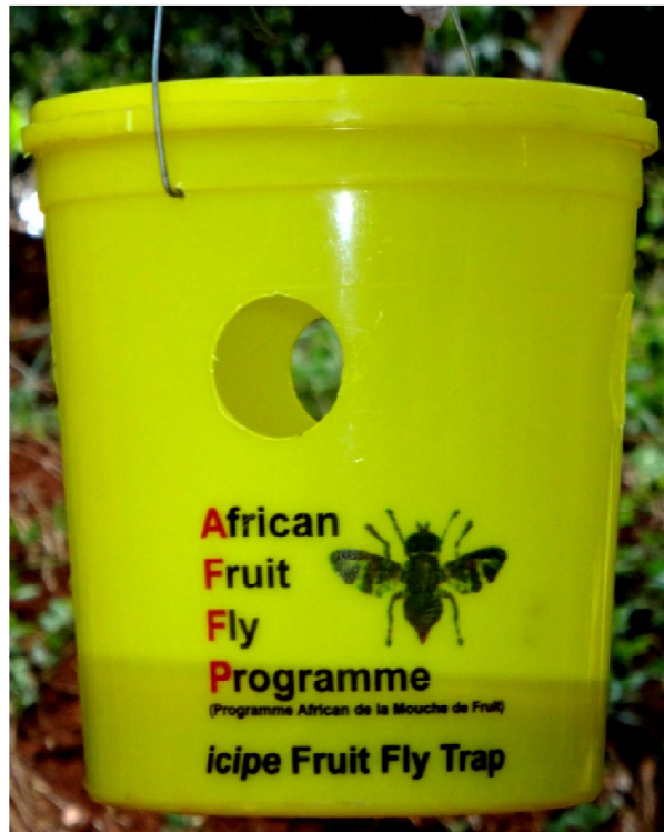
Figure 3.2: Lynfield trap with 250 ml of Dudulure fruit fly bait for monitoring fruit fly population in the field.
