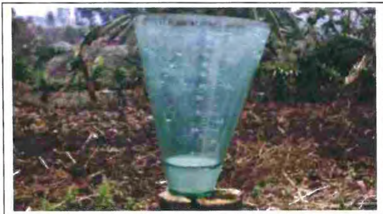
Plate 3.6: Rain gauge for recording rainfall
