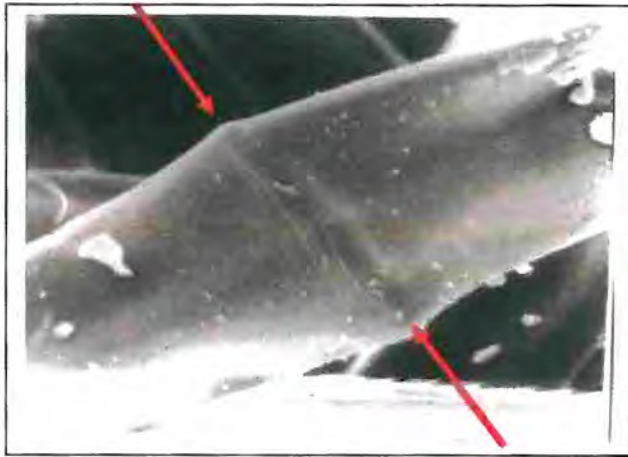
Plate 7.5: SEM of a brin of A. panda silk fibre showing the bamboo joint (arrows)
