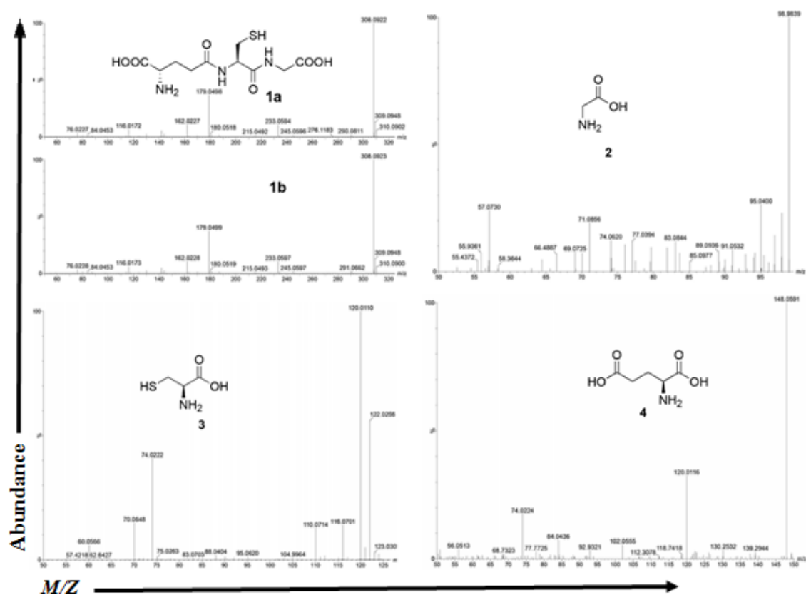
Figure 4.6: Representative mass spectrum showing (1a) natural GSH, (1b) synthetic GSH, (2) glycine, (3) cysteine and (4) glutamic acid
