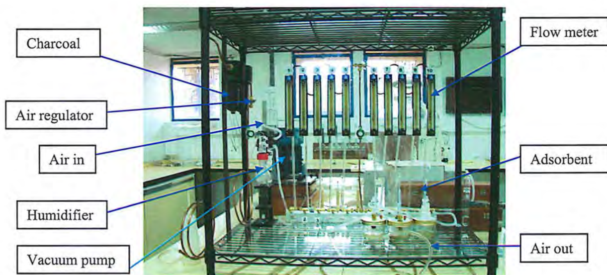
Plate 3.1. Dynamic volatile collection system.
