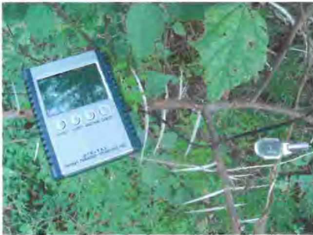
Plate 5.5 Digital in/outdoor thermo-hygrometer in Imba forest
