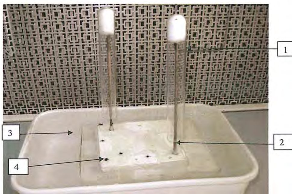
Plate 4. 1: Experimental arena made up of inverted glass tubes (Nana, 2009)
