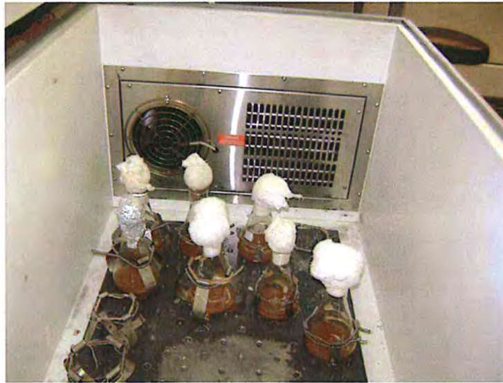
Plate 3. 2: Starter cultures of M. anisopliae in orbital shaker incubator (Ouna, 2009)
