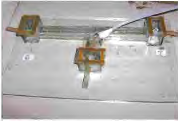
Figure 4.1 Two-choice olfactometer. (Air is passed over the left and right chambers containing the source of volatiles by sucking air out of the front central chamber containing the ticks)
