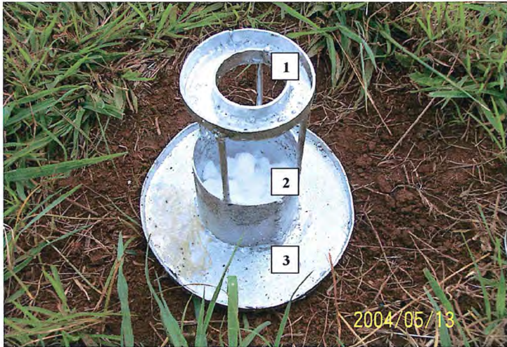
Plate 6.1: Trap set in the field, carrying AAAP and 1-octen-ol (1), CO 2 (2) and Neem Cake Extracts (3).
