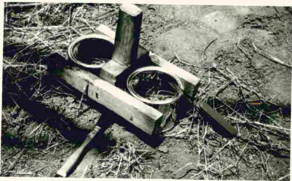
Plate 1: A photograph of the apparatus (two open-ended tins) used for sampling un-foraged grass litter (arrow 1) and foraged grass litter (arrow 2) and foraging soil of Odontotermes .
